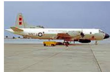
VW4 was flying P3 aircraft at the time it decommissioned. There were 4 P3 modified with heavier landing gear and the electronics were upgraded for weather work with an onboard weather station and the infamous APS 20 search radar. The radome was installed in the bomb bay and was capable of being lowered and raised.
